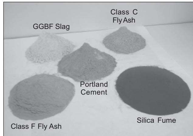
has cementitious properties by itself but these are enhanced when it is used with portland cement. Slag is used at 20% to 70% by mass of the cementitious materials.
